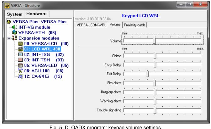
Fig. 5. DLOADX program: keypad volume settings.
