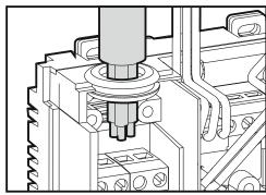
10. Screw the 230 V AC power leads to the corresponding terminals (phase conductor to L terminal, neutral conductor to N terminal, and protective conductor to PE terminal).
