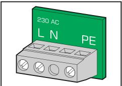
11. Screw the wire fastening element.
