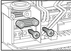
9. Run the cable through the cable grommet.
