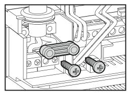
12. Replace the cover of power supply terminals.
