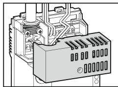
13. Replace the screw fastening the cover of power supply terminals.
