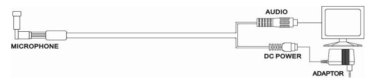
Remark: Since Hi sensitivity microphone, MIC001 audio pick up box must be put at 5 meters away from monitor to avoid any audio reverberation.
