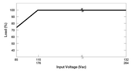
No output power de-rating for the input voltage from 115Vac to 132Vac & 176Vac to 264Vac
