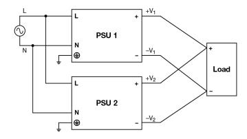
Fig. 6 Parallel Operation Connection Diagram
